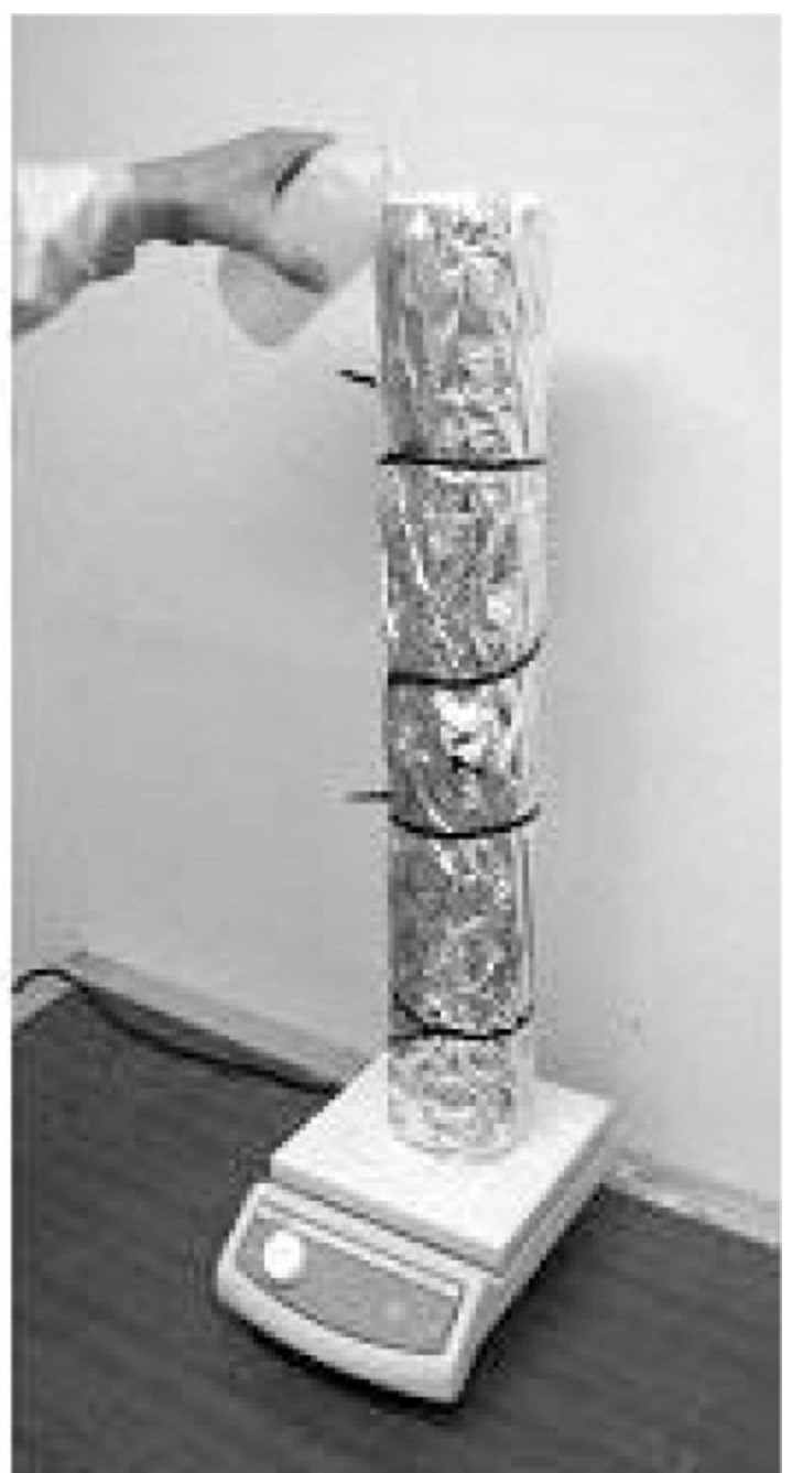
FIGURE 2 Wet Insulation Cyclic Testing Apparatus (180°C – 450°C)
