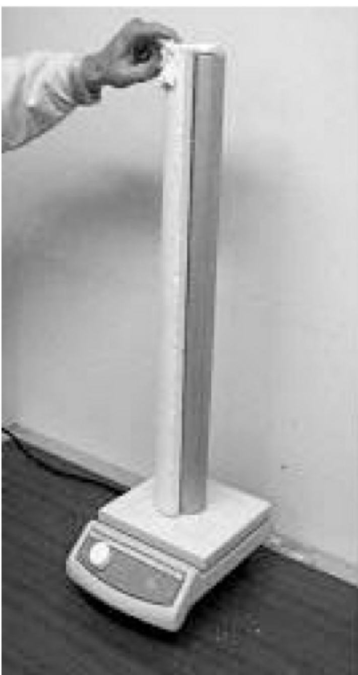
FIGURE 2 Wet Insulation Cyclic Testing Apparatus (180°C – 450°C)
