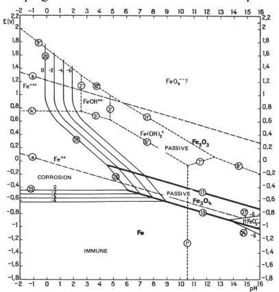
**FIGURE 1.1**. — Potential pH equilibrium diagram for the system iron-water, at 25 C (considering as solid substances only Fe, Fe30, and Fe203).
