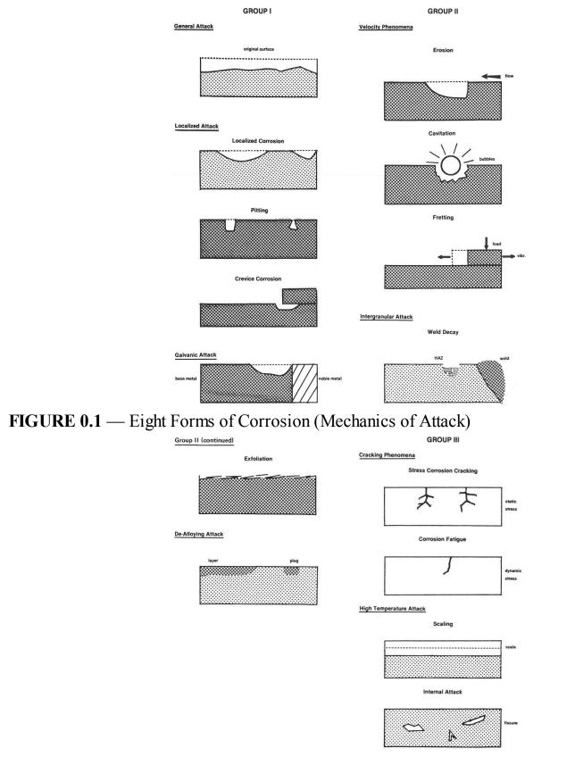
FIGURE 0.1 — Eight Forms of Corrosion (Mechanics of Attack) Continued
